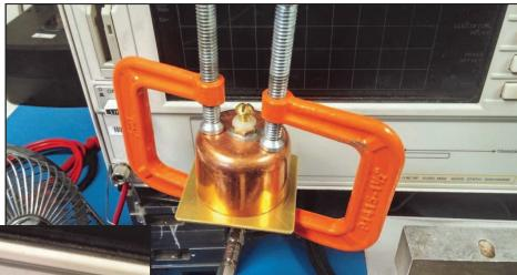
As you can see, Doug includes real craftsmanship in his builds. The SMA connectors are the kind with Teflon sleeves (used to pass through machined housings). I wonder if the exposed nuts have any effect on the filter characteristics?
